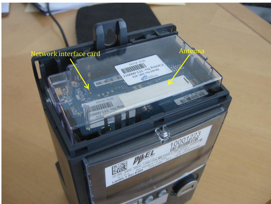
The Smart Meters operate in a mesh network. Metering information is fed back to a nearby access point either directly, or by being relayed through one or more other meters in the network.
