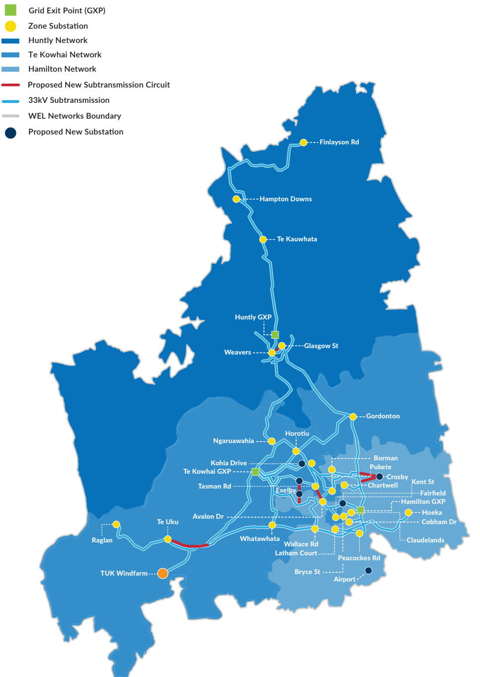
Figure 6.1.2.1: Overview of the WEL Network System
