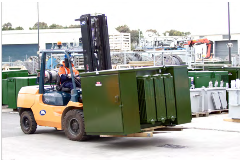
Photo 16 500kVA Groundmount Transformer being moved in the Distribution Centre
