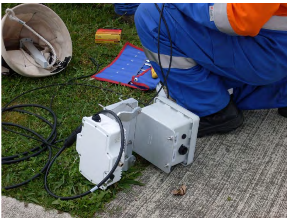
Photo 17 Smart Box relay prior to being installed on a pole
