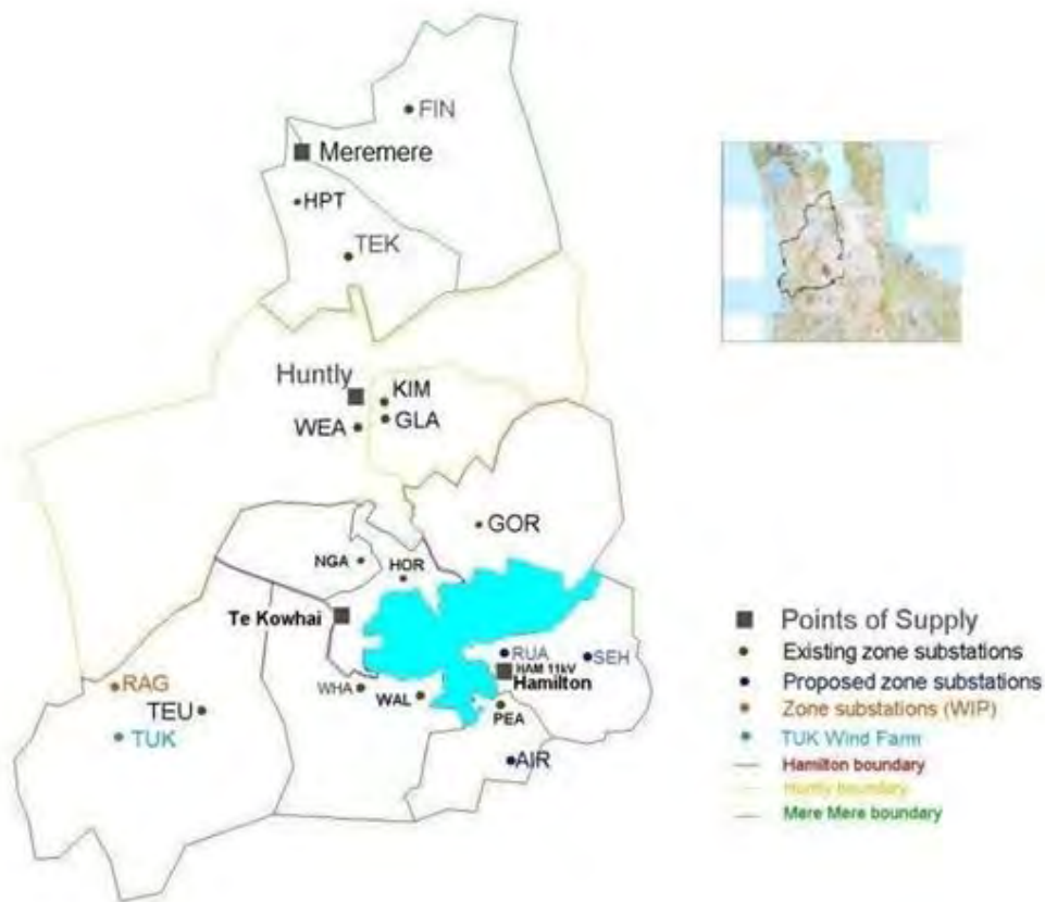
Figure 15. Points of Supply, existing zone substations, associated supply zones and proposed zone substations.
